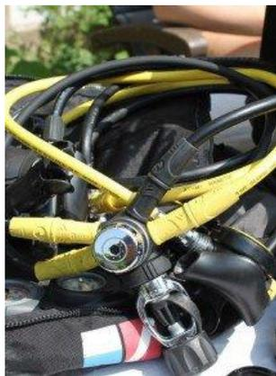
Check your regulator set visually by pulling back on any hose protectors you may have, and ensure that all hoses are intact and haven't started cracking at the points where they bend.
