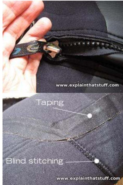
Photo: Above: A tough brass zip and thickened rubber flaps keep water out of the back of this winter wetsuit. Below: This is what a wetsuit looks like inside. The outer neoprene is lined with smooth nylon (which feels better on your skin). The seams of the suit are blind-stitched and taped to stop cold water getting in and warmed water getting out.
